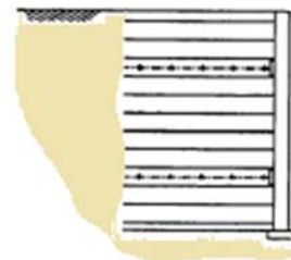
Full-Height Concrete Panel
