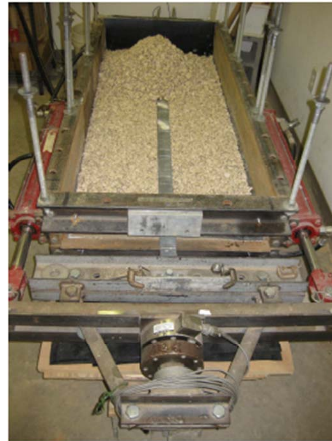
Figure 3. Setup of RECO 2" wide galvanized steel strip pullout test within 570-1" crushed limestone.
